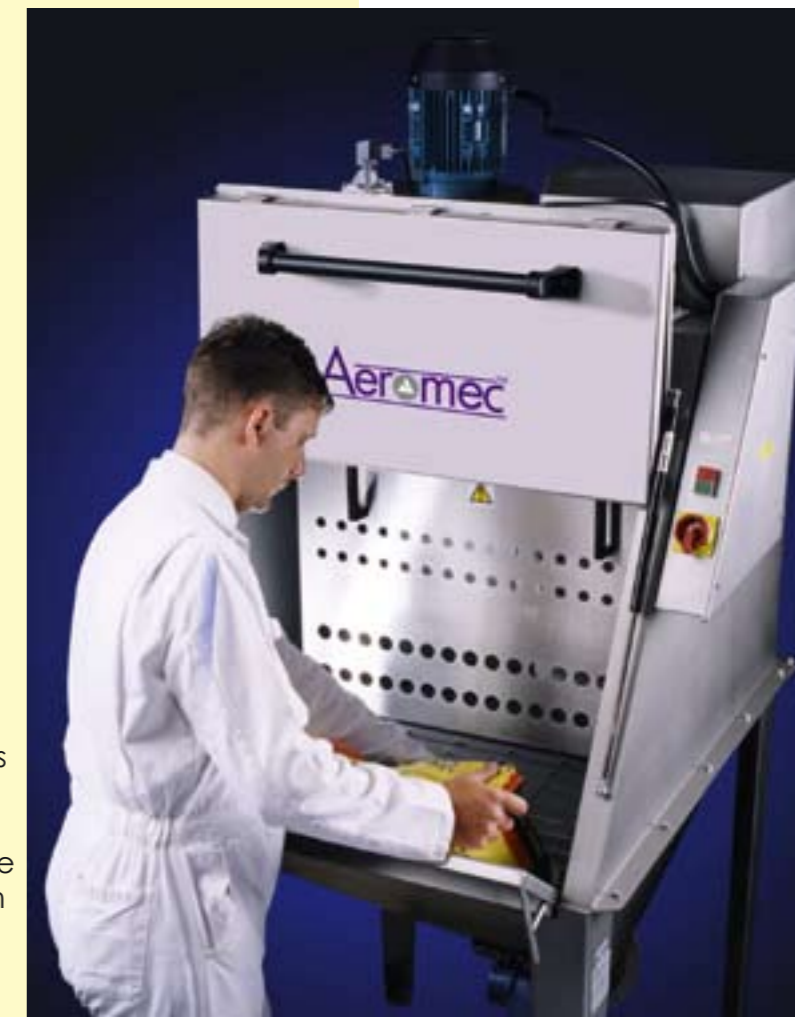
Sack tip station discharging into a 1000 litre powder mixer manufactured by Entecon UK Ltd
