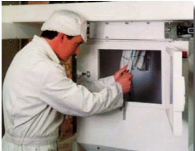
Operator untying neck of FIBC
