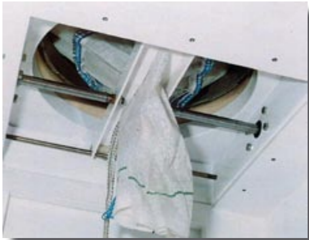
Knife valve in closed position sealing neck of FIBC
